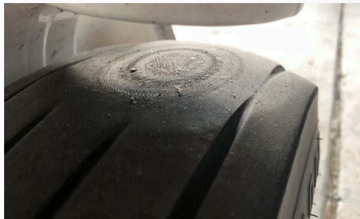
The Problem: FlatSpots can cause heavy breaking issues and lead to skidding meanwhile the landing an breaking process
